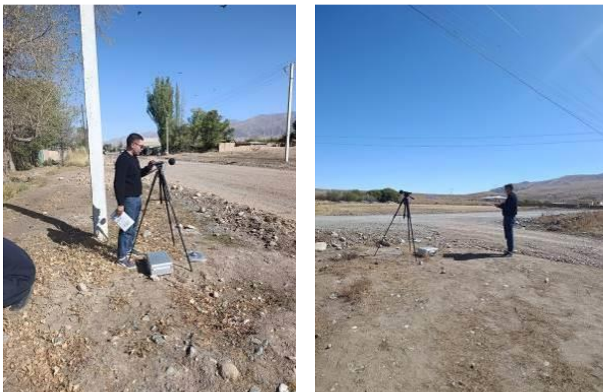
Figure 29: Instrumental monitoring of noise and vibration levels
